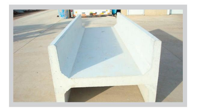
Our deep H bunks come in 10' lengths and are 3 1/2" thick throughout. Side heights are at 30" and overall width is 42" across. Feed area is 36" across and 14" deep. This bunk weighs 3,650 lbs.
